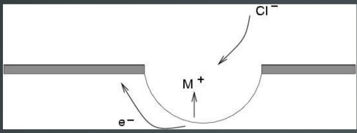
mechanism of pitting corrosion
